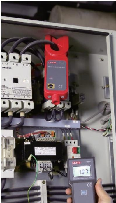
UT255 series high voltage clamp ammeters can measure up to 69kV high voltage line current and leakage current. UT255 comes with an insulation rod, allowing professional users to check status of lightning arresters. The wireless model (UT255B) is also able to wirelessly transmit data in real-time up to 30m range. Its clamp can be easily removed from wire by pressing or pulling back the insulation rod.
