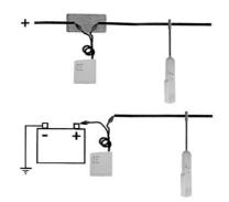
Press and hold down the measurement key on the receiver and follow the signal and thus the cable with the sensor.
